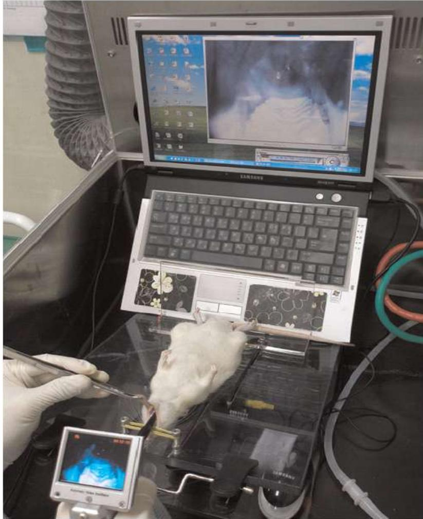
Figure 3 A photograph of a charged-coupled device video image that is displayed simultaneously on the liquid-crystal display screen of the automatic video instillator and on a computer monitor at the time of intratracheal instillation of a 0.25% (w/v) solution of Evans Blue dye
