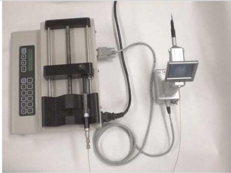
Figure 2 Photograph of the tubing and cable connection between the automatic video instillator and the syringe pump
