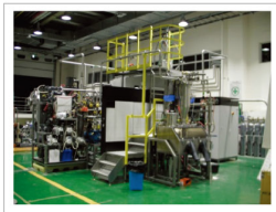
Atmosphere control (control of carrier gas's oxygen concentration), oxygen/Ar mixed gas used
