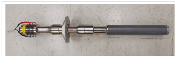
BLT for ultrasonic casting of pistons
