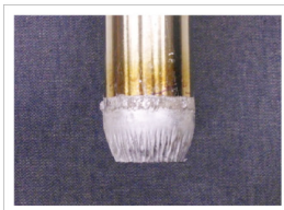
Cavitation erosion on metal tip
