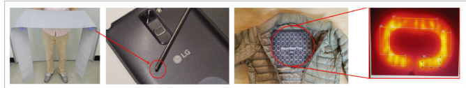
Al textile electrode material and stylus pen and wearable heating pad using it
