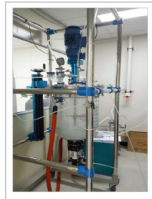
Production system for Al precursor ink material (50L/batch)
