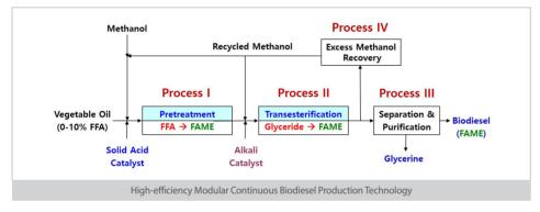
Continuous modular biodiesel production process that modularizes each of its sub-processes, including oil
