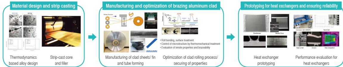
Manufacturing high performance, thin-walled clad for brazing and improving reliability of heat exchanger components
